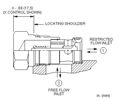
This valve is a fixed-orifice, non-pressure-compensated flow control with a reverse flow check. The flow setting is specified by the user and is set at the factory.
