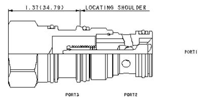
Free-flow, side-to-nose cheater check valves with a bypass orifice function as a 2-port check valve in a 3-port cavity. They allow free flow from port 2 to port 1 with a customer specified orifice that controls flow from port 1 to port 2. Port 3 of the cartridge is blocked off.
