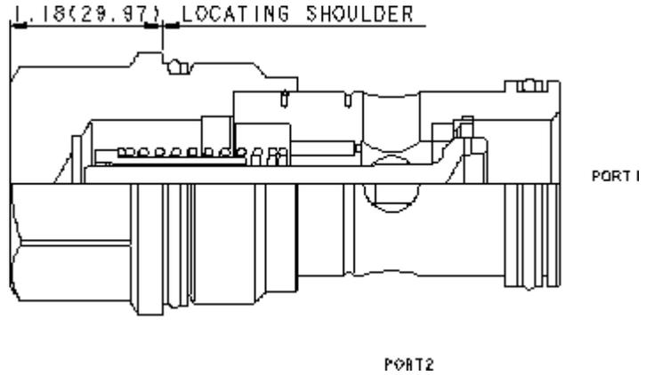
This valve is a fixed-orifice, non-pressure-compensated flow control with a reverse flow check. The flow setting is specified by the user and is set at the factory.
