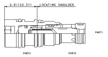
This valve is a spring biased closed, pilot-to-close check cartridge that has a 1.8:1 pilot ratio. The valve allows flow from port 1 to port 2 and blocks reverse flow. Pressure at the pilot port opposes pressure at port 1 at a ratio of 1.8:1. This valve is most often used in regeneration circuits.
