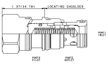
This valve is a spring biased closed, pilot-to-close check cartridge that has a 1.8:1 pilot ratio. The valve allows flow from port 1 to port 2 and blocks reverse flow. Pressure at the pilot port opposes pressure at port 1 at a ratio of 1.8:1. This valve is most often used in regeneration circuits.
