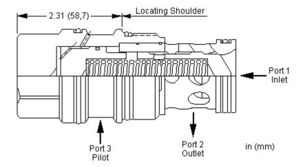
This valve is a spring biased closed, pilot-to-close check cartridge that has a 1.8:1 pilot ratio. The valve allows flow from port 1 to port 2 and blocks reverse flow. Pressure at the pilot port opposes pressure at port 1 at a ratio of 1.8:1. This valve is most often used in regeneration circuits.
