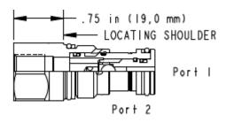
The single ball shuttle connects the higher of two work ports to the signal or common port. The signal is sensed at an
