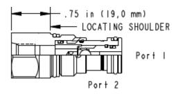
The single ball shuttle connects the higher of two work ports to the signal or common port. The signal is sensed at an
