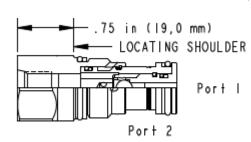
The single ball shuttle connects the higher of two work ports to the signal or common port. The signal is sensed at an
