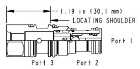
The single ball shuttle connects the higher of two work ports to the signal or common port. The signal is sensed at port 3.
