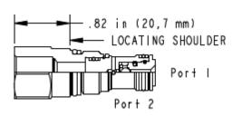
The single ball shuttle connects the higher of two work ports to the signal or common port. The signal is sensed at an external port located in the hex-end of the cartridge.
