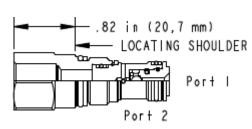
The single ball shuttle connects the higher of two work ports to the signal or common port. The signal is sensed at an external port located in the hex-end of the cartridge.
