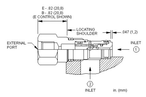
The single ball shuttle connects the higher of two work ports to the signal or common port. The signal is sensed at an external port located in the hex-end of the cartridge.
