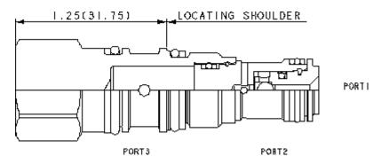
The single ball shuttle connects the higher of two work ports to the signal or common port. The signal is sensed at port 3.
