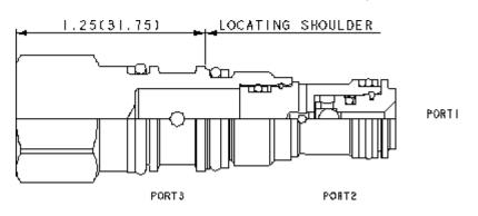
The single ball shuttle connects the higher of two work ports to the signal or common port. The signal is sensed at port 3.
