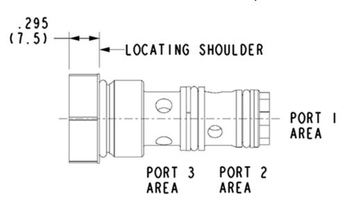
The single ball shuttle connects the higher of two work ports to the signal or common port. The signal is sensed at port 2.
