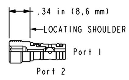
The single ball shuttle connects the higher of two work ports to the signal or common port. The signal is sensed at port 2.
