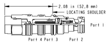
This valve is a pilot to open check valve. It has a sealed pilot, a steel seat, and is vented. It allows free flow from the valve (port 2) to the load (port 1) and blocks flow in the opposite direction. Pressure at the pilot (port 3) will open the valve from port 1 to port 2. Pilot pressure needed to open the valve is directly proportional to the load pressure at port 1. The valve is insensitive to pressure at port 2 because the spring chamber is referenced to the vent (port 4).
