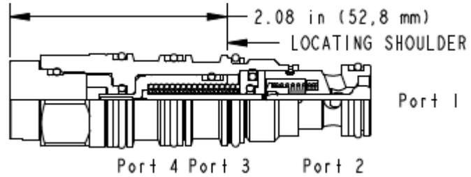
This valve is a pilot to open check valve. It has a sealed pilot, a steel seat, and is vented. It allows free flow from the valve (port 2) to the load (port 1) and blocks flow in the opposite direction. Pressure at the pilot (port 3) will open the valve from port 1 to port 2. Pilot pressure needed to open the valve is directly proportional to the load pressure at port 1. The valve is insensitive to pressure at port 2 because the spring chamber is referenced to the vent (port 4).
