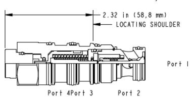
This valve is a pilot to open check valve. It has a sealed pilot, a steel seat, and is vented. It allows free flow from the valve (port 2) to the load (port 1) and blocks flow in the opposite direction. Pressure at the pilot (port 3) will open the valve from port 1 to port 2. Pilot pressure needed to open the valve is directly proportional to the load pressure at port 1. The valve is insensitive to pressure at port 2 because the spring chamber is referenced to the vent (port 4).
