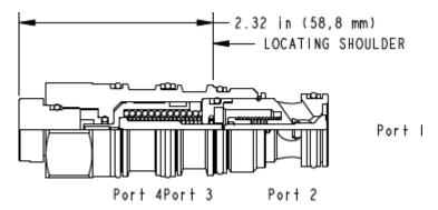
This valve is a pilot to open check valve. It has a sealed pilot, a steel seat, and is vented. It allows free flow from the valve (port 2) to the load (port 1) and blocks flow in the opposite direction. Pressure at the pilot (port 3) will open the valve from port 1 to port 2. Pilot pressure needed to open the valve is directly proportional to the load pressure at port 1. The valve is insensitive to pressure at port 2 because the spring chamber is referenced to the vent (port 4).
