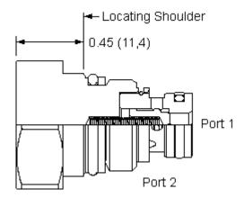
Free-flow, nose-to-side check valves are on/off circuit components that allow free flow from the inlet (port 1) to the outlet (port 2) and block flow in the opposite direction.
