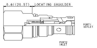
Free-flow, side-to-nose check valves are on/off circuit components that allow free flow from the inlet (port 2) to the outlet (port 1) and block flow in the opposite direction.
