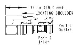
Free-flow, side-to-nose check valves are on/off circuit components that allow free flow from the inlet (port 2) to the
