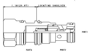
Free-flow, side-to-nose cheater check valves function as a standard 2-port check valve in a 3-port cavity with port 3 of the cartridge blocked off. These valves are useful in circuits where a check valve is required in an existing three port cavity.
