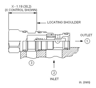
Free-flow, side-to-nose cheater check valves function as a standard 2-port check valve in a 3-port cavity with port 3 of the cartridge blocked off. These valves are useful in circuits where a check valve is required in an existing three port cavity.
