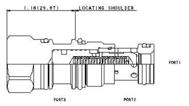
Free-flow, nose-to-side cheater check valves function as a standard 2-port check valve in a 3-port cavity with port 3 of the cartridge blocked off. These valves are useful in circuits where a check valve is required in an existing three port cavity.
