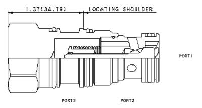
Free-flow, side-to-nose cheater check valves function as a standard 2-port check valve in a 3-port cavity with port 3 of the cartridge blocked off. These valves are useful in circuits where a check valve is required in an existing three port cavity.
