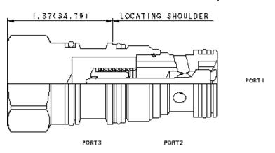
Free-flow, side-to-nose cheater check valves function as a standard 2-port check valve in a 3-port cavity with port 3 of the cartridge blocked off. These valves are useful in circuits where a check valve is required in an existing three port cavity.
