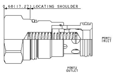
Free-flow, nose-to-side check valves are on/off circuit components that allow free flow from the inlet (port 1) to the outlet (port 2) and block flow in the opposite direction.
