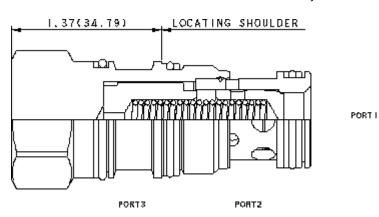
Free-flow, nose-to-side cheater check valves function as a standard 2-port check valve in a 3-port cavity with port 3 of the cartridge blocked off. These valves are useful in circuits where a check valve is required in an existing three port cavity.
