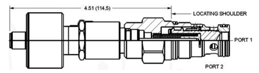
Free-flow, nose-to-side check valves are on/off circuit components that allow free flow from the inlet (port 1) to the outlet (port 2) and block flow in the opposite direction. This valve incorporates a position switch to provide confirmation that the valve is in the transition position or seated (closed).
