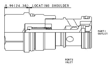
Free-flow, side-to-nose check valves are on/off circuit components that allow free flow from the inlet (port 2) to the outlet (port 1) and block flow in the opposite direction.
