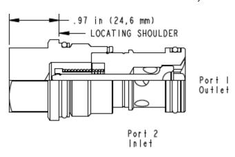
Free-flow, side-to-nose check valves are on/off circuit components that allow free flow from the inlet (port 2) to the outlet (port 1) and block flow in the opposite direction.
