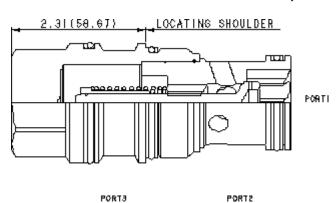
Free-flow, side-to-nose cheater check valves function as a standard 2-port check valve in a 3-port cavity with port 3 of the cartridge blocked off. These valves are useful in circuits where a check valve is required in an existing three port cavity.
