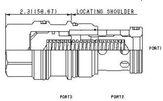
Free-flow, nose-to-side cheater check valves function as a standard 2-port check valve in a 3-port cavity with port 3 of the cartridge blocked off. These valves are useful in circuits where a check valve is required in an existing three port cavity.
