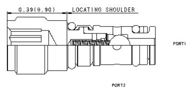
Free-flow, nose-to-side check valves are on/off circuit components that allow free flow from the inlet (port 1) to the outlet (port 2) and block flow in the opposite direction.
