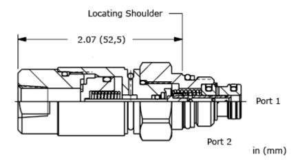
These pilot-stage, directional, 2-position, 2-way valves are pneumatically operated, spring-return cartridges and are available in either normally open or normally closed configurations. These cartridges are designed for pilot flow applications and utilize Sun's T-8A cavity so they can be used in conjunction with Sun's pilot-operated, main-stage valves.
