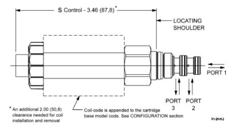
This solenoid-operated 3-way, 2-position cartridge is a direct-acting, balanced spool pilot valve used to pilot other full-flow valves. The valve is normally open between port 1 and port 2 or port 1 and port 3 and all flow paths are bidirectional. This valve is designed to be used with 740 and 747 Series coils.
