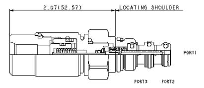
These pilot-stage, directional, 2-position, 3-way valves are hydraulically operated, spring-return cartridges and are available in two spool configurations; normally open 1 to 2 and normally open 1 to 3. These cartridges are designed for pilot flow applications.
