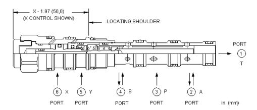
Three-position, 4-way directional cartridges are spring-centered, 6-port directional valves that can be configured from a choice of spool options. The supply port is port 3 and all ports will accept 5000 psi (350 bar). Capacity for these pilot-to-shift valves is dependent on the spool type specified.
