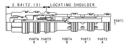
Two-position, detented, 4-way directional cartridges are 6-port directional valves that can be configured with up to 3 different spool options. The supply port is port 3 and all ports will accept 5000 psi (350 bar). Capacity for these pilot-to-shift valves is dependent on the spool type specified.
