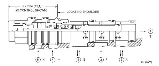
Two-position, 4-way directional cartridges are spring-offset, 6-port directional valves that can be configured from a choice of 9 different spool options. The supply port is port 3 and all ports will accept 5000 psi (350 bar). Capacity for these pilot-to-shift valves is dependent on the spool type specified.
