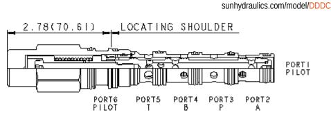
Three-position, 4-way directional cartridges are springcentered, 6-port directional valves that can be configured
