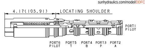
Three-position, 4-way directional cartridges are spring-centered, 6-port directional valves that can be configured from a choice of spool options. The supply port is port 3 and all ports will accept 5000 psi (350 bar). Capacity for these pilot-to-shift valves is dependent on the spool type specified.
