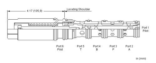
Three-position, 4-way directional cartridges are spring-centered, 6-port directional valves that can be configured from a choice of spool options. The supply port is port 3 and all ports will accept 5000 psi (350 bar). Capacity for these pilot-to-shift valves is dependent on the spool type specified.
