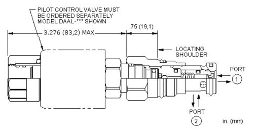
This valve is a 2-position, 2-way poppet cartridge that incorporates an integral pilot control cavity. It controls flow from port 1 to port 2, exhibits extremely low leakage rates and will accept 5000 psi (350 bar) at both ports. Installing a pilot solenoid cartridge in the T-8A cavity results in a high-flow directional valve. Other pilot options include manual, hydraulic and pneumatic pilot cartridges.
