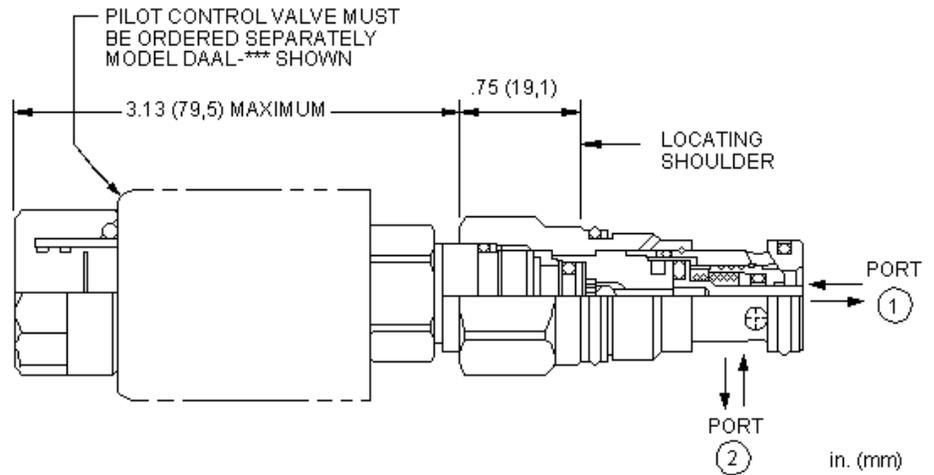
This valve is a 2-position, 2-way poppet cartridge that incorporates an integral pilot control cavity. It controls flow from port 2 to port 1, exhibits extremely low leakage rates and will accept 5000 psi (350 bar) at both ports. Installing a pilot solenoid cartridge in the T-8A cavity results in a high flow directional valve. Other pilot options include manual, hydraulic and pneumatic pilot cartridges.
