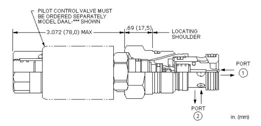
This valve is a 2-position, 2-way poppet cartridge that incorporates an integral pilot control cavity. It controls flow from port 1 to port 2, exhibits extremely low leakage rates and will accept 5000 psi (350 bar) at both ports. Installing a pilot solenoid cartridge in the T-8A cavity results in a high-flow directional valve. Other pilot options include manual, hydraulic and pneumatic pilot cartridges.
