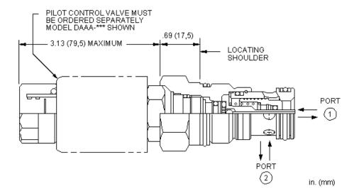
This valve is a 2-position, 2-way poppet cartridge that incorporates an integral pilot control cavity. It controls flow from port 2 to port 1, exhibits extremely low leakage rates and will accept 5000 psi (350 bar) at both ports. Installing a pilot solenoid cartridge in the T-8A cavity results in a high flow directional valve. Other pilot options include manual, hydraulic and pneumatic pilot cartridges.
