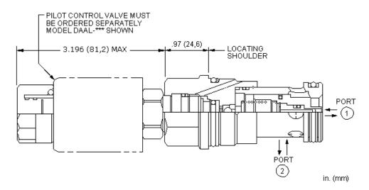
This valve is a 2-position, 2-way poppet cartridge that incorporates an integral pilot control cavity. It controls flow from port 1 to port 2, exhibits extremely low leakage rates and will accept 5000 psi (350 bar) at both ports. Installing a pilot solenoid cartridge in the T-8A cavity results in a high-flow directional valve. Other pilot options include manual, hydraulic and pneumatic pilot cartridges.
